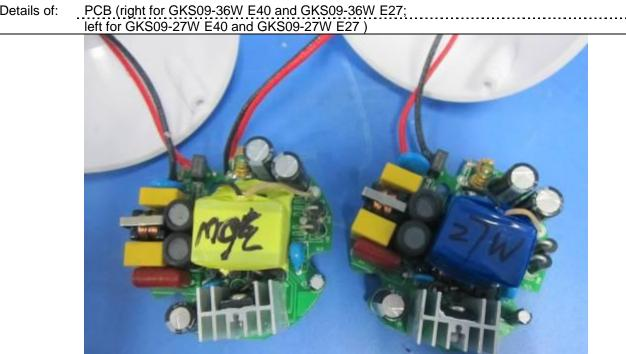
PCB layout (right for GKS09-36W E40 and GKS09-36W E27; left for GKS09-27W E40 and GKS09-27W E27 ) Details of:
