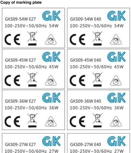
Location: sticking on the external enclosure of lamp. (Height of letters and numerals at least 2mm, Height of WEEE mark at least 7mm, height of CE mark at least 5mm.)
